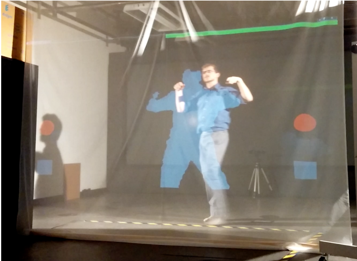
Figure 7.5: The FOOT system UI. The red circles on either side are the record buttons, and the lower grey squares are the library buttons. The green rectangle overhead is the stage occupancy indicator, showing that the current user is on the right side of the stage.
