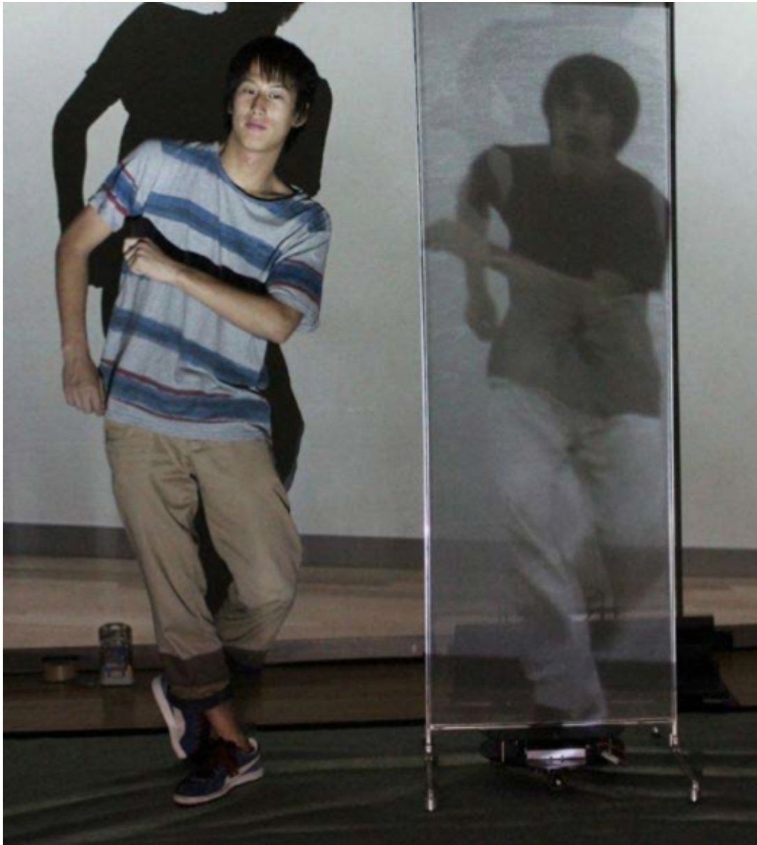
Figure 3.2: The work of Tsuchida et al., showing a live dancer alongside a self-propelled robot with a projection screen on top. A calibrated projector projects the video of a pre-recorded dancer on the screen [Tsuchida et al., 2013].
