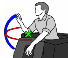
Figure 2. A resting elbow (green X) creates a pivot point and can only access 2 degrees of freedom (red and blue arcs), even through a 3-d space.
